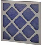
These high quality disoposable filters consist of cardboard frames and lattice facings. The non-woven filtration medium is bonded to coarse mesh supports then pleated to give an extended face area and minimise resistance. The pleated pack is then encased within the disposable cardboard frame.
