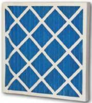
High quality disposable filters consist of cardboard frames and lattice facings. The medium is graduated spun glass or synthetic, depending on efficiency requirements. The media is then encased within a cardboard frame.
