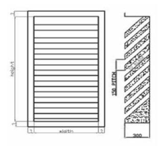
Louvre Weights Approx 50kg/M<sup>2</sup>-Galvanised 35kg/M<sup>2</sup>-55kg/M<sup>2</sup>-Stainless
